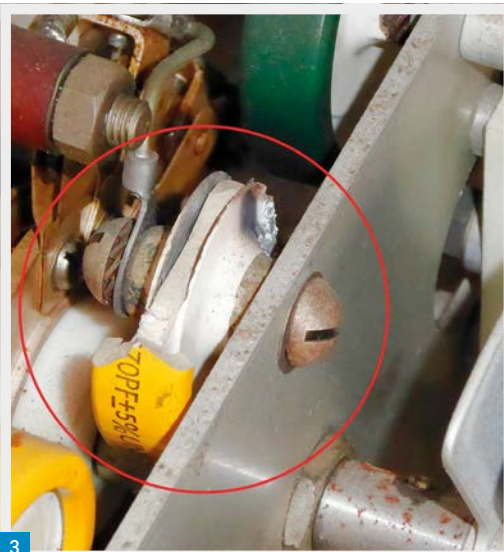
Fig. 3: Damaged antenna load capacitor. Fig. 4: Fault monitoring board.
