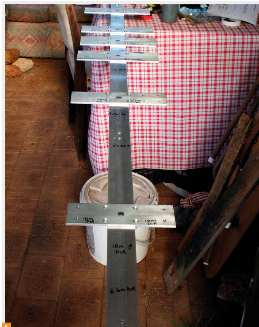
Fig. 4: XR6 boom marked ready for adding elements. Fig. 5: XR6 boom with element mounting plates in place.
