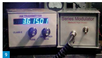
Fig. 8: LCD or LED options for reading frequency.
